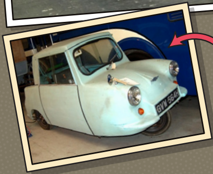
Invacar from the 1970s – Invacars were a type of vehicle designed for disabled drivers. They had 3 wheels and could only seat the person driving the car.
